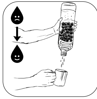
② Filter water with charcoal and cloth
