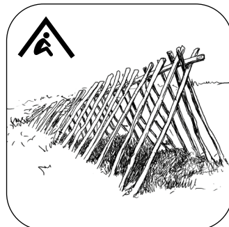
⑬ Make an "A" frame as a base for shelter
